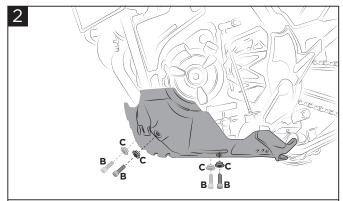
Secure the Acerbis skid plate (A) using the provided bushings (B) and screws (C).
