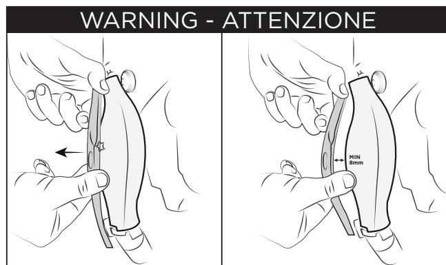
**If it's not possible to have a minimum distance from the exhaust pipe of 8mm, it is possible to deform the protection, tighten the clamps where the protection hole is aligned and then tighten the screw.**
