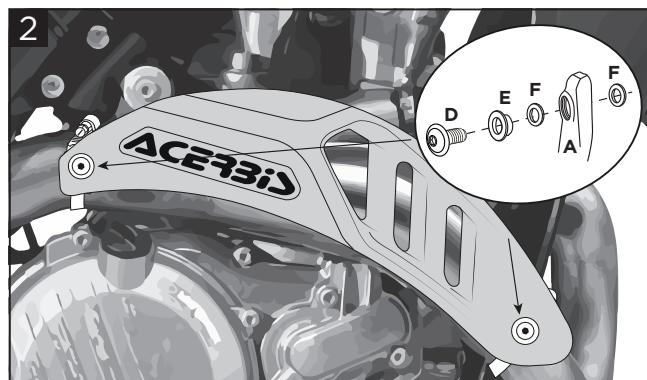
**Attach the head shield (A) with the supplied bolt (D), bushing (E) and washers (F) as shown in figure. Tighten loosely.**
