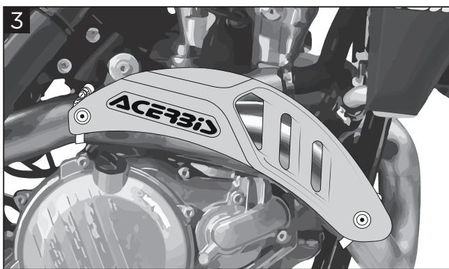
**Arrange the shield and clamps so that the shield is a minimum of 8 mm away from the exhaust pipe and tighten the clamps (B). Then tighten the head shield to the clamps and torque to 4Nm. After one hour of use, check the tightness of the clamps and shield and tighten if needed.**
