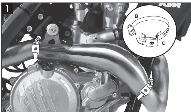
**Insert the threaded plates (C) into the hose clamps (B) and then attach to the muffler loosely.**
